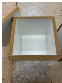
Figure 2: Insulated moulds with samples size 100mm 3 and insulation of 50mm
