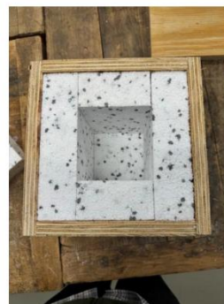
Figure 2: Insulated moulds with samples size 100mm 3 and insulation of 50mm
