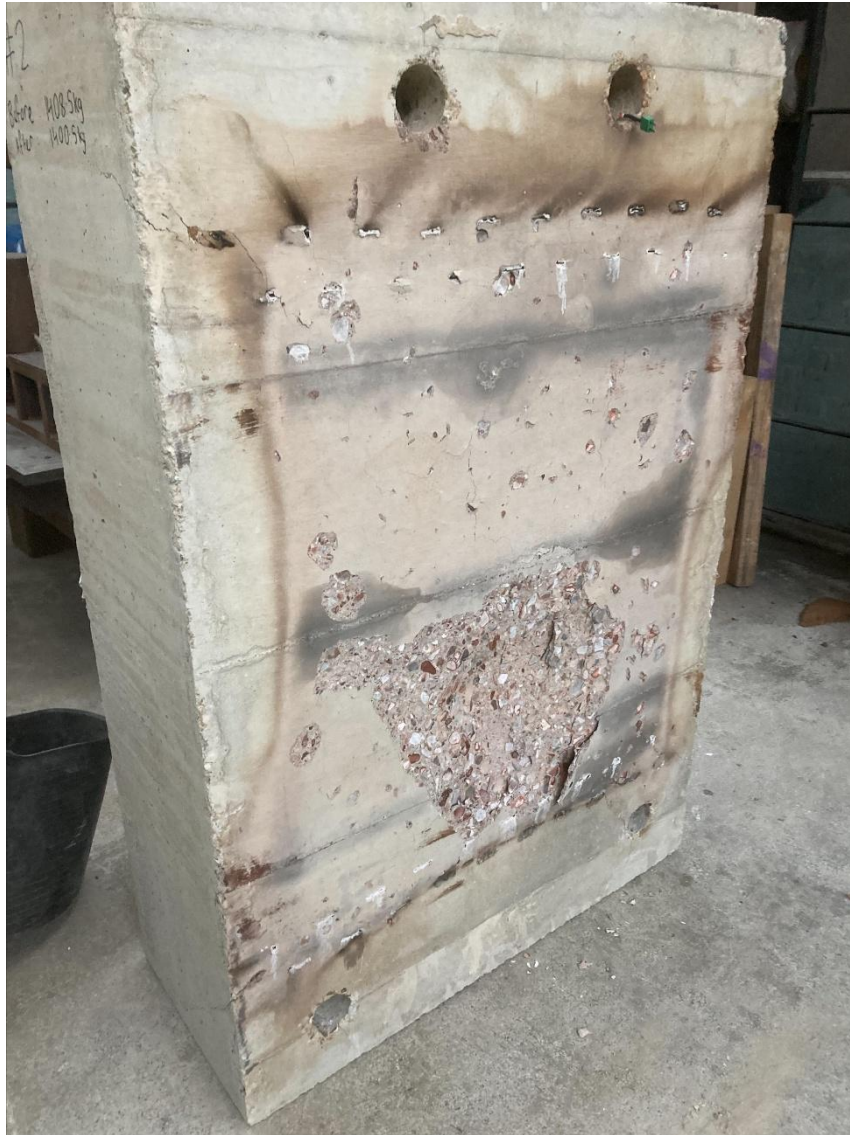
Figure 2. ACT specimen after testing showing minor spalling
