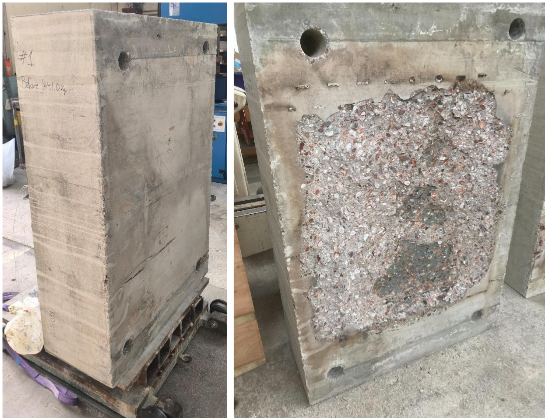
Figure 4. Conventional concrete specimen before (left) and after (right) fire testing
